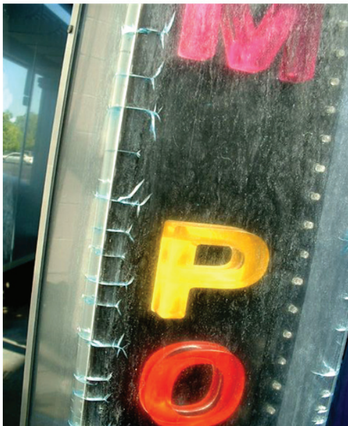
EXAMPLE 1. THIS SIGN FACE WAS CLEANED WITH WINDEX OR CAR WASH CHEMICALS CAUSING IT TO CRACK.
